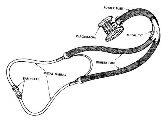
Figure 5-3. Stethoscope.
